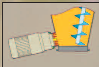
High speed choppers are added to many Vertical Blender designs to accelerate the blending process by breaking down lumps.
