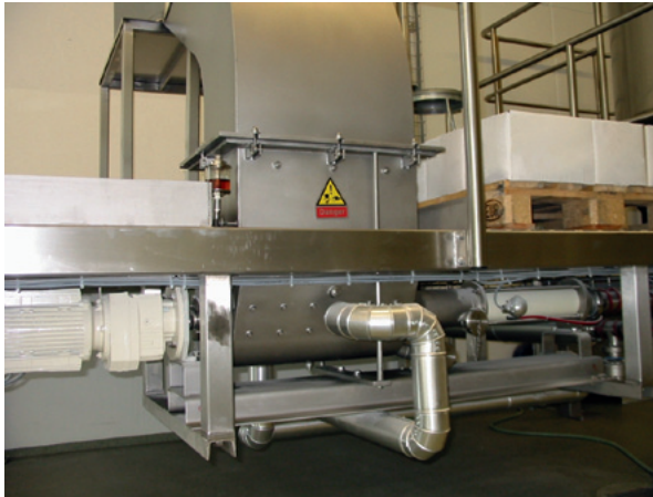
seepex pump range BTCS with heatable double-jacket design
